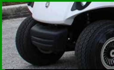
You know and we know: things happen out there. So we made our bumpers with thicker walls and textured surfaces to withstand mishaps. They're the same height front and rear to minimize damage. They release air on impact; in fact, they're 5 mph rated.
