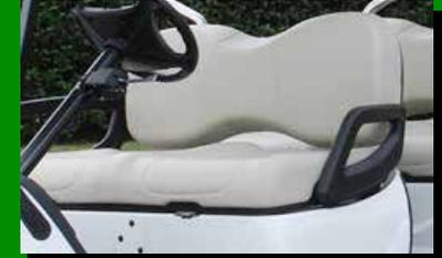
Deep, supportive contours provide unmatched comfort. The widest seat in the industry is designed to accommodate occupants of different heights and sizes. Its made of pure, supple foam bonded to a seamless, durable vinyl backed cover and its polypropylene seat.
